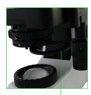
Swing-out filter holder in condenser for color adjustment provides easy access.
