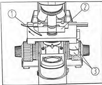
**2. Placing the Specimen Slide**
