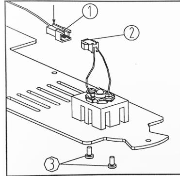
6. Remove the two screws, indicated by the red arrows, that hold the LED assembly plate. Remove the LED assembly from base and detach wires.
